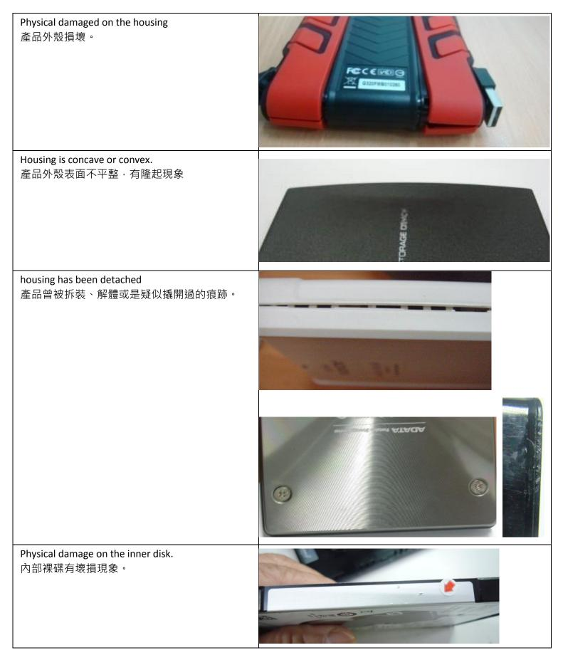
Physical induced damaged in the inner disk / Inner disk has concave or convex mark. 內部裸碟變形。
