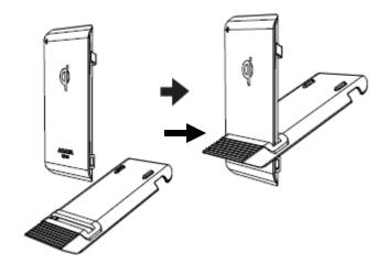
iii. b. Depending the phone's orientation, size, and induction zone position, adjust the upper and lower covers to the most appropriate location.
