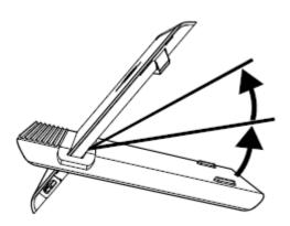
iv. Confirm that the metal cover plate is in flat contact with the charging cover and that the bases are level, in order to maintain the charging stand stability.
