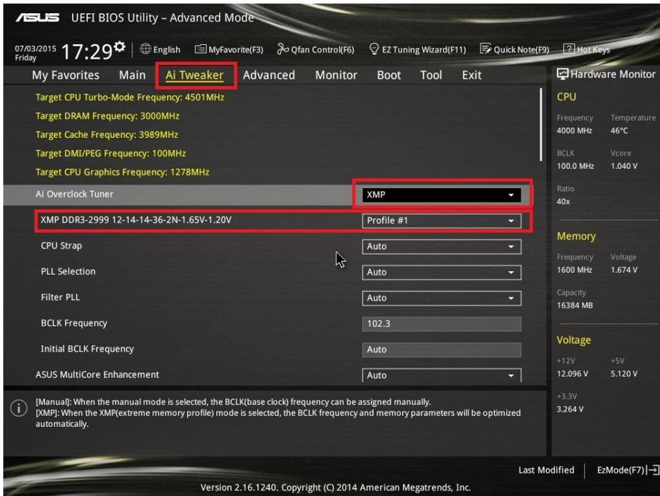
After confirming that these are the settings you want, press F7 to exit Ai Tweaker and F10 to save and restart your PC for XMP settings to take effect. As before, on restarting re-enter the BIOS to make sure overlocking has been applied.
