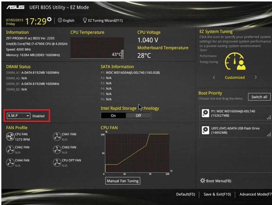
Based on the XMP parameters supported by the installed memory, you can load available XMP pre-sets such as Profile 1 as shown, using the drop menu.
